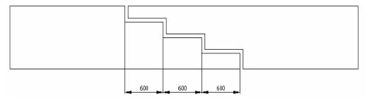
Fig. 1. One way of preparing the conveyor belt ends
