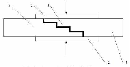
Fig. 2. Flow diagram of combining ply rubber carpet:1 - belts conveyor which will be submitted to junction process,2 - electric plates, 3 - rubber ATRBZ
